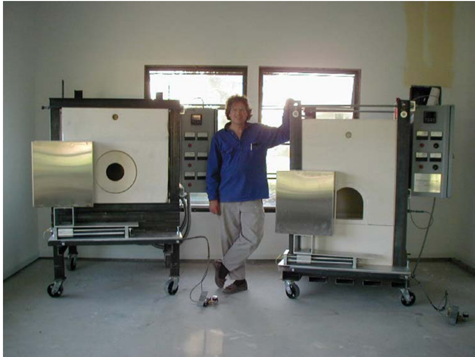
Glory Hole 1624 with reducing ring – 175-Pound capacity Furnace
