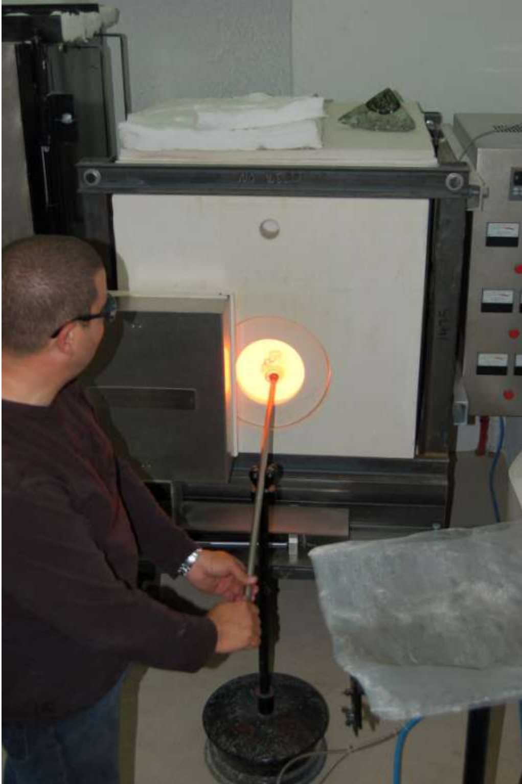
Dcampana Glass Studio, Calvi, Corsica, France – All Electric Studio™ Dominique Campana Working with the Glory Hole
