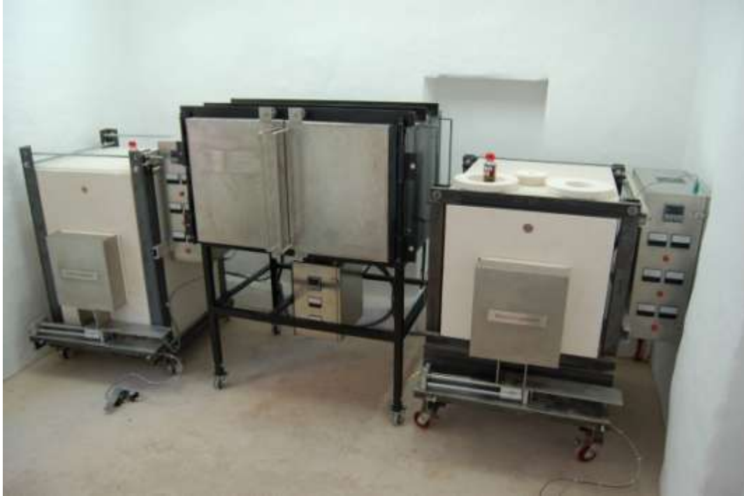
Dcampana Glass Studio, Calvi, Corsica, France – All Electric Studio™ Electroglass® Furnace 250-B, Annealer FL-483624, Glory Hole
