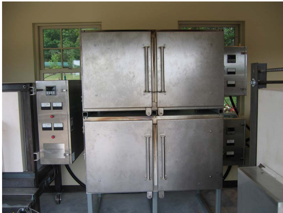
Glory Hole 1616 (left) - Stacked Electroglass ® Annealers – Furnace (right)
